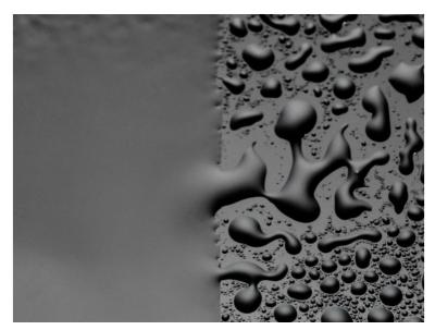
Comparison of the anti-stick and easy-to-clean effect of the uncoated (left) with the coated side (right).
